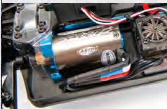
Wasserfester Brushless Antrieb/ Waterresistant Brushless combo 12T/3300KV + 45 A Brushless Controller
