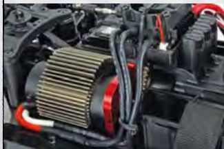
Der wasserfeste Dragster 4S Brushless-Antrieb (1980 UpV) / The water resistant DRAGSTER 4S Brushless-Combo (1980 kv)
