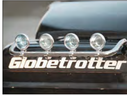
Lampenbügel Volvo aus vernickeltem Messing Volvo lamp frame made of nickel-plated brass N° 500907076
